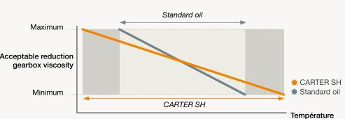
The technology used to formulate **CARTER SH** provides stable performance in extreme service conditions. Its wide operating temperature range makes it ideal for lubricating numerous types of industrial transmissions.
