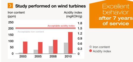
**CARTER SH** ensures extended lifetime both for the oil and lubricated mechanical parts.
